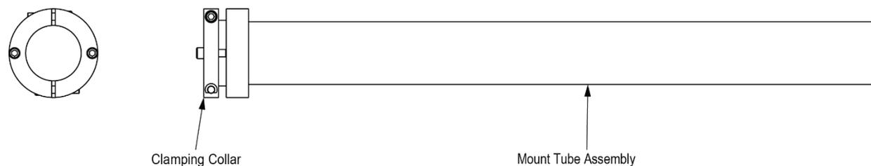
Figure 1-2 Typical DuraFire Mounting Tube
